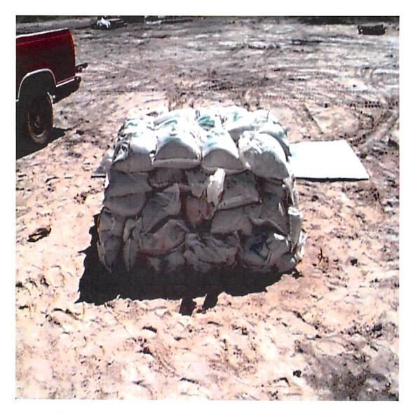
Figure 5 – Sandbag Enclosure for an 81 mm M374A2 mortar
