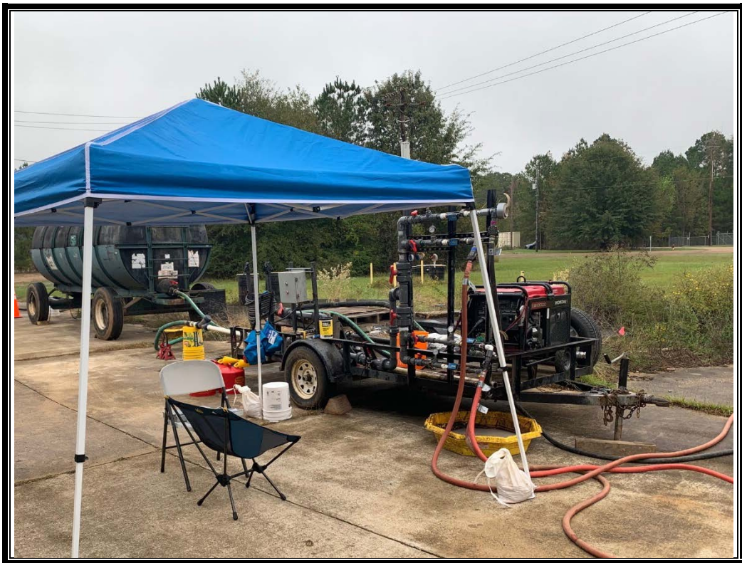
PHOTO 1: Injection Trailer and Mobile 4,000-gallon Tank at LHAAP-04 DATE: October 28, 2019
